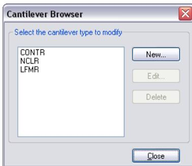
The cantilever browser dialog is opened via the menu 'Options>Config Cantilever Types...'. The cantilever browser allows the editing and creation of cantilever types.
