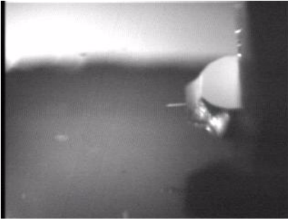
Side view of the cantilever after manual coarse approach
