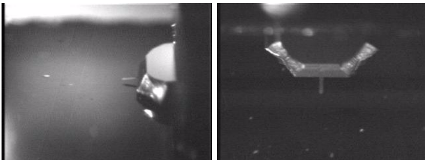
View of the cantilever after manual approach: left: side view, right: top view
