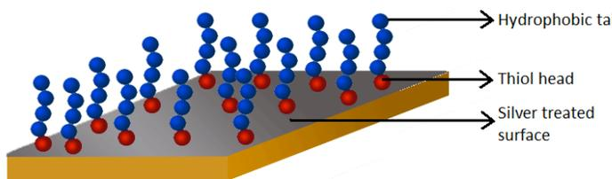
Figure 2. Self assembled monolayer made of HDFT molecules.
