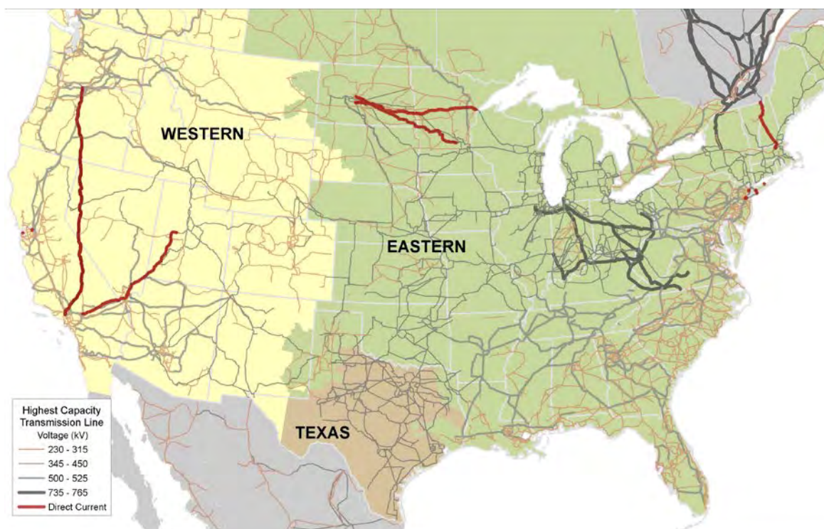
Figure 2-12. Transmission systems and three main grid interconnections in North America
