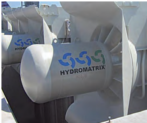
Source: Andritz Hydro Figure 1-10. Modular application of standard turbine runners to an existing dam
