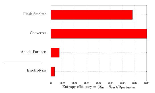
Figure 23: The Second Law efficiency of copper production is incredibly small. The steps in sorting the copper atoms are: Ore Concentration  $2\% \rightarrow 30\%$  Cu (not shown); Smelter  $30\% \rightarrow 63\%$  Cu; Converter  $63\% \rightarrow 99.1\%$  Cu; Anode furnace  $99.1\% \rightarrow 99.55\%$  Cu; and Electrolysis  $99.55\% \rightarrow 99.99\%$  Cu. Source: STEFAN GÖSSLING, Entropy Production as a Measure for Resource Use, University of Hamburg, 2001.
