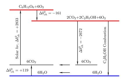
Figure 41: Exergy diagram of the ideal CO<sub>2</sub>-Glucose-EtOH cycle.
