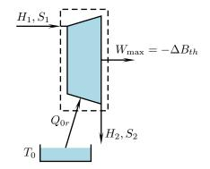
Figure 32: Exergy balance in an isothermal, ideal flow machine. The maximum possible shaft work from this machine is equal to the negative change of thermal exergy.
