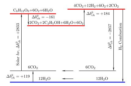
Figure 42: Exergy diagram of the ideal CO<sub>2</sub>-Glucose-EtOH-H<sub>2</sub> cycle.
