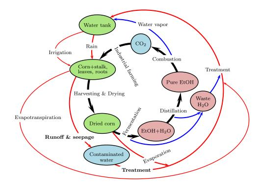
Figure 40: The water cycle in corn-ethanol production. Compared with the water requirement by corn plants, the feed water requirement of an ethanol-producing plant is small, and the link between the tank and the fermentation stage was not drawn. Adapted from Figure 7 in BERTHIAUME et al. (2001).
