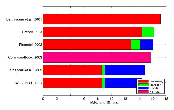
Figure 18: The average fossil energy inputs to ethanol production in a wet milling plant. The length of each bar is the total energy outlay to produce 1 liter of EtOH, and the blue parts denote the size of energy credits assumed by the different authors. The modern dry mill plants use 11.36 MJ/L as steam and 3.12 MJ/L as electricity, 14.5 MJ/L total, not counting transportation costs.
