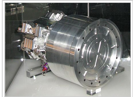
A Flybrid Systems Kinetic Energy Recovery System built for use in Formula One
