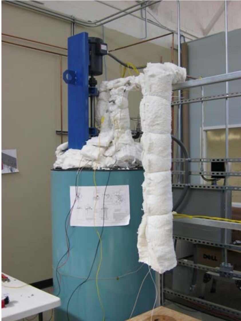
Figure 11. Picture of the Cold Tank including the pump mounted on the lid.
