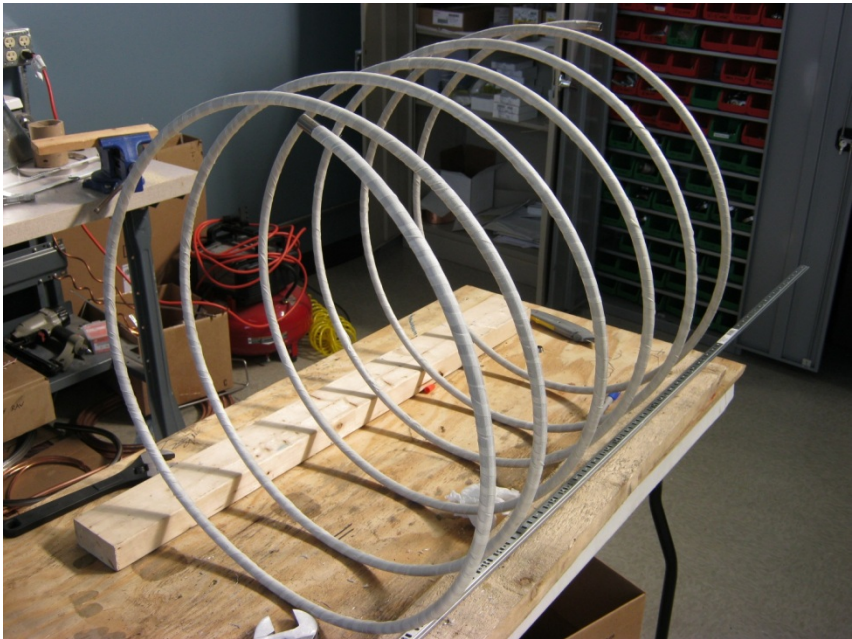
Figure 34. Insulation tape is wrapped around the tubing prior to wrapping the electrical heating tape for the second version.
