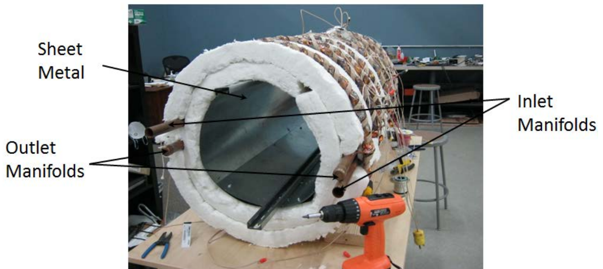
Figure 38. The manifolds are attached, insulation is added, and sheet metal completes the interior assembly of the HX.
