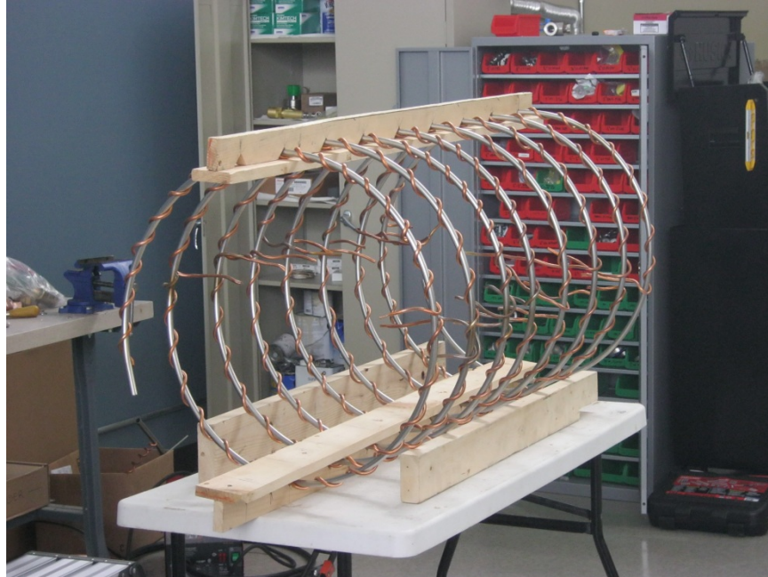
Figure 37. The copper tubing is wound around the salt coiled (steel) tubing. The ends of the copper tubing are visible and then fit into the ½ inch copper manifolds.
