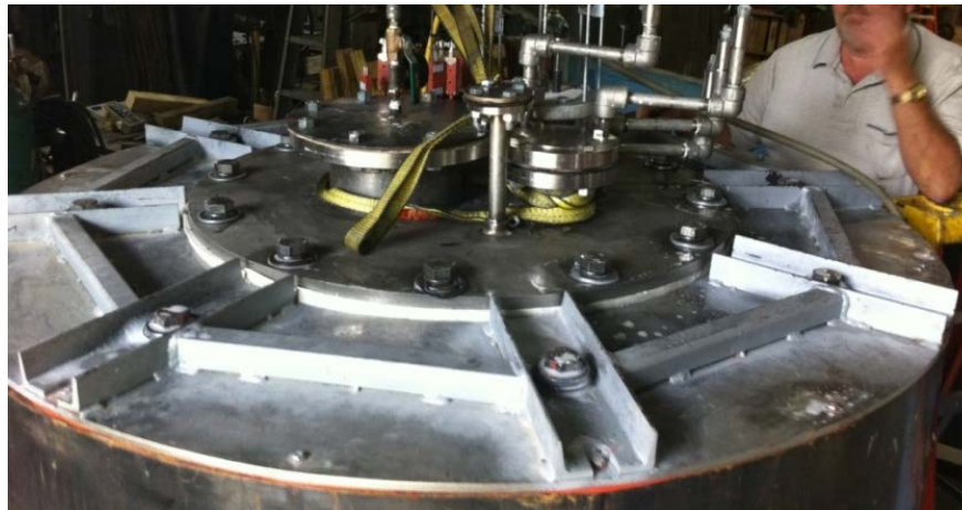
Figure 25. The lid is assembled for leak testing.
