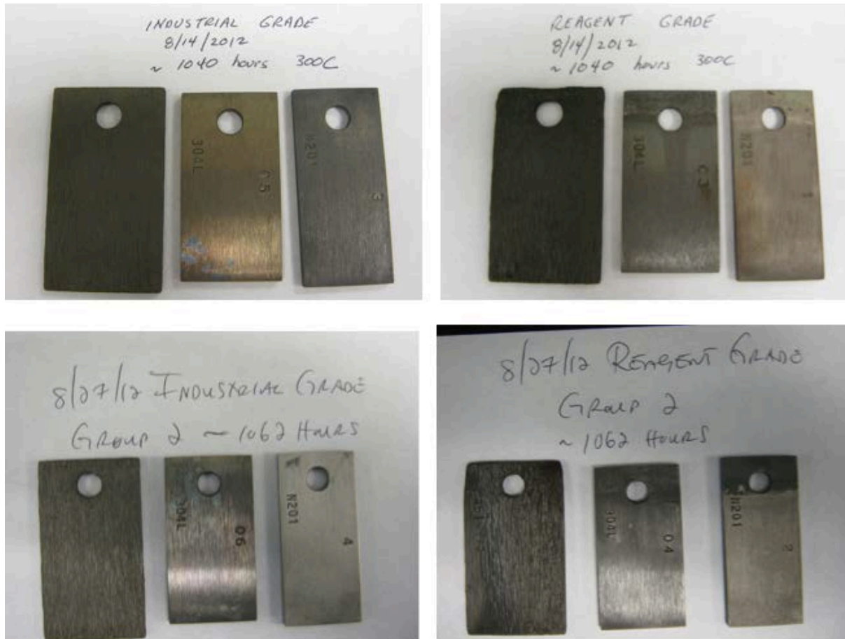
Figure 53. Appearance of corrosion coupons after approximately 1000 hours in Industrial grade or Reagent grade Saltstream700 at 300°C. In each photo, the order is A516, 304L, Nickel 201 from left to right.
