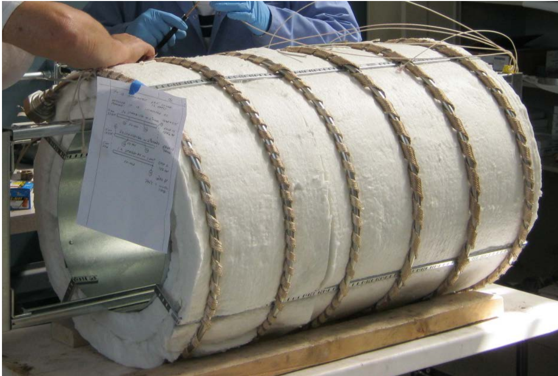
Figure 32. Construction of the FX. Heating tape is wrapped around stainless steel coiled tubing. The coil is encased in Fiberfrax insulation.
