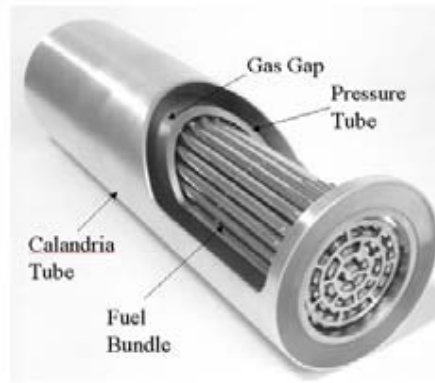
FIG. X-4. Current CANDU fuel channel.
