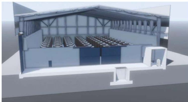
FIG. 2. 70 casks can be stored in the SFDS (Krško NPP archive) (reproduced from Ref. [5] with permission).
