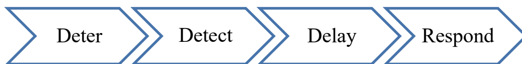
FIG. 2. Security system functions.
