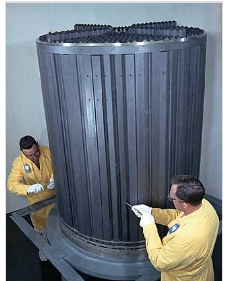
Core graphite from the Molten-Salt Reactor Experiment
