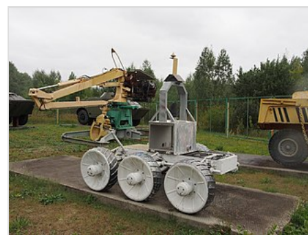
STR-1 robot used in cleanup, nicknamed "Moon Walker"
