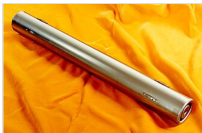
An N Reactor fuel rod. It consists of metallic uranium assemblies (two concentric cylinders with zirconium cladding) 66 centimetres (26 in) long and 6 centimetres (2.4 in) in diameter. The uranium enrichment is 1.25 percent.
