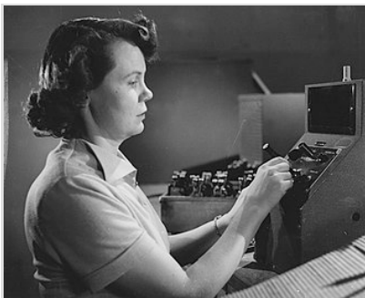
As part of regular health physics procedures, a laboratory assistant checks a pocket ionization chamber at a minometer.
