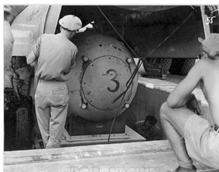
A pumpkin bomb (Fat Man test unit) being raised from the pit into the bomb bay of a B-29 for bombing practice during the weeks before the attack on Nagasaki
