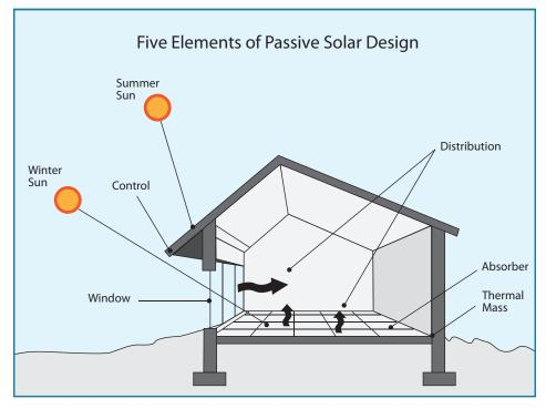
5. Control – Elements such as roof overhangs or trees can be used to shade the window during summer months. Other elements for controlling temperature include electronic sensing devices, such as differential thermostats that signal a fan to turn on, vents and dampers that allow or restrict heat flow, low-emissivity (low-e) blinds, and awnings.
