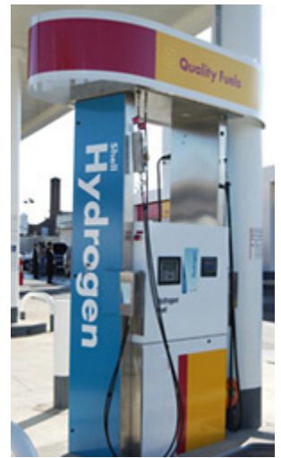
Hydrogen fueling pump
