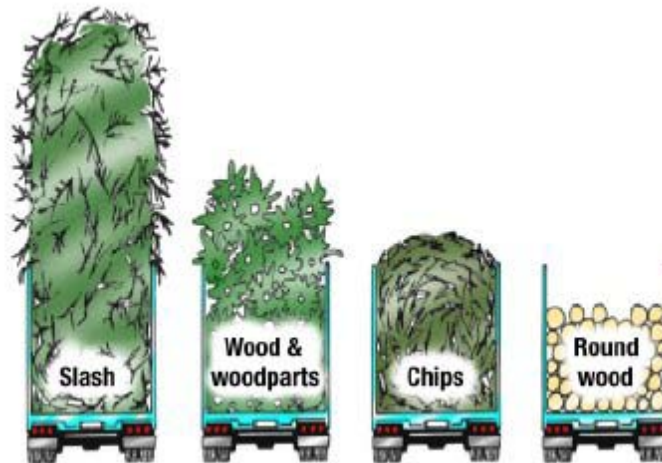
Figure 4.3.1. Bulk volume of woody biomass in different processed forms with the same weight (Hubbard, Biles, Mayfield, and Ashton, 2007)
