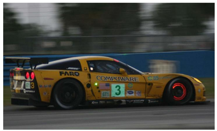
Without regenerative braking, cars turn excess speed into heat using brakes, as can be seen by the glowing brake rotor in this picture. Flickr/Freewheeling Daredevil
