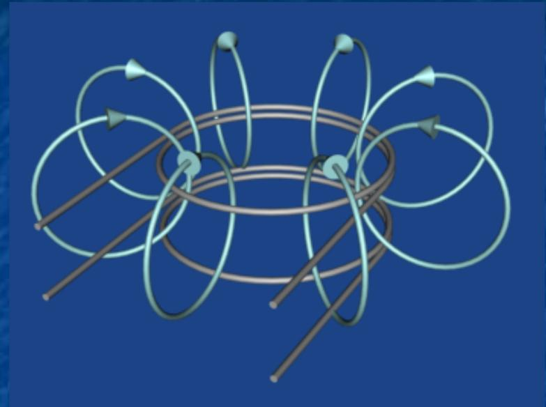
Side view: **See how growing field from top coil sweeps thru the lower coil!**
