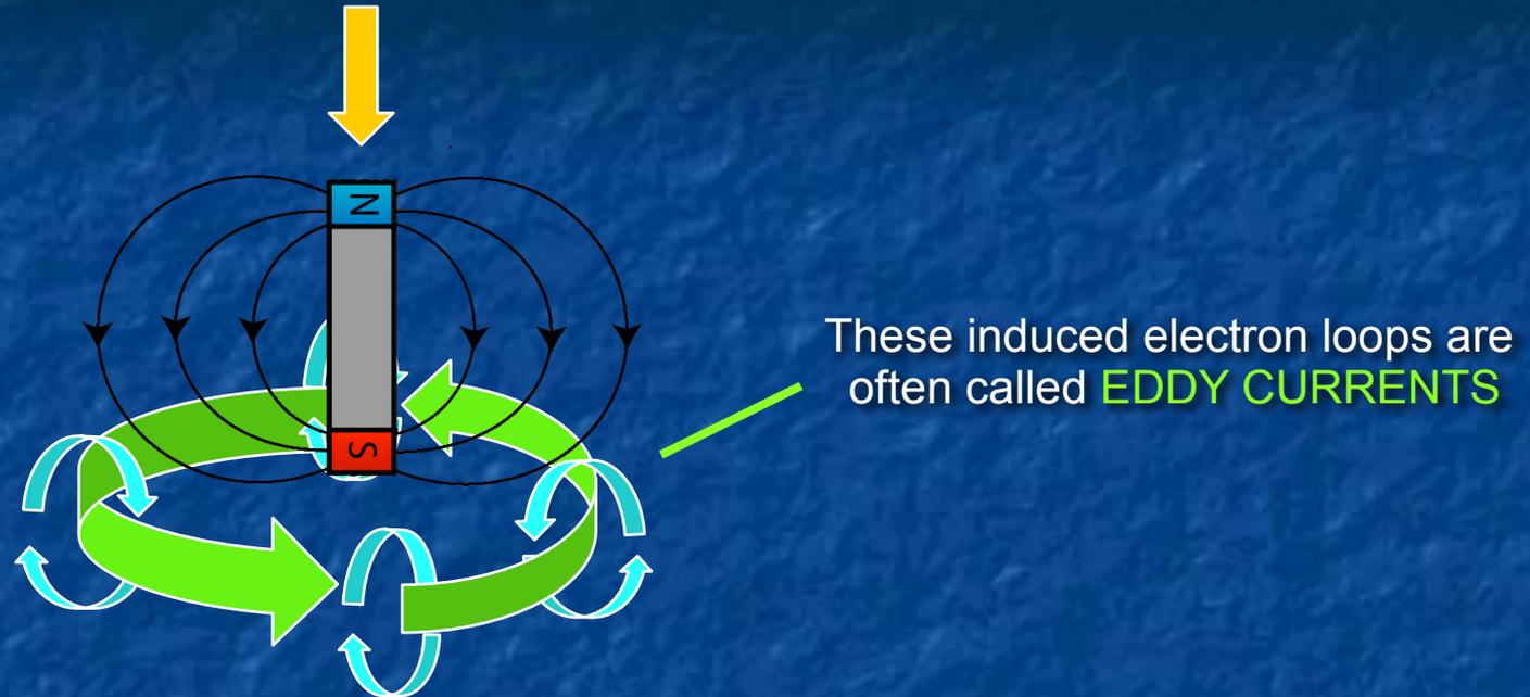
**Electro-Magnetism** then causes the **electron loop** to produce its own **magnetic field**
