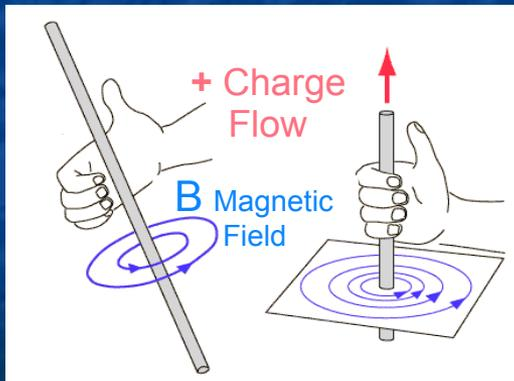
Thumb in direction of **+ charge** flow,
