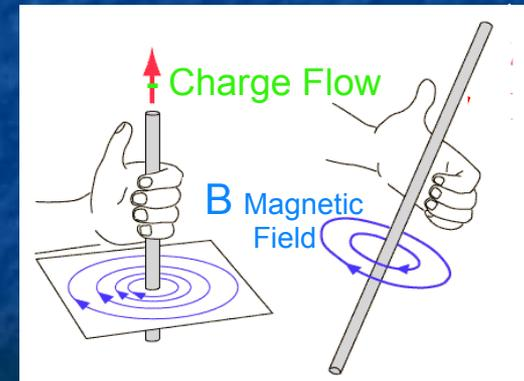
Thumb in direction of **- charge** flow.
