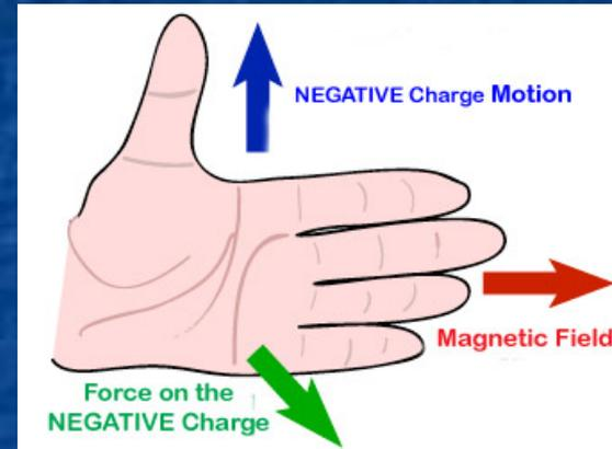
"MOTION" = Part of electron's velocity that is perpendicular to the magnetic field
