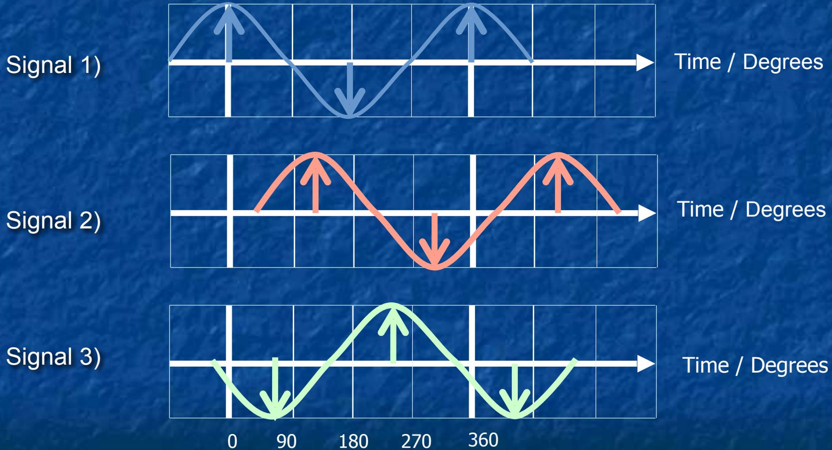
Arrows mark when each AC power signal reached an up or down peak
