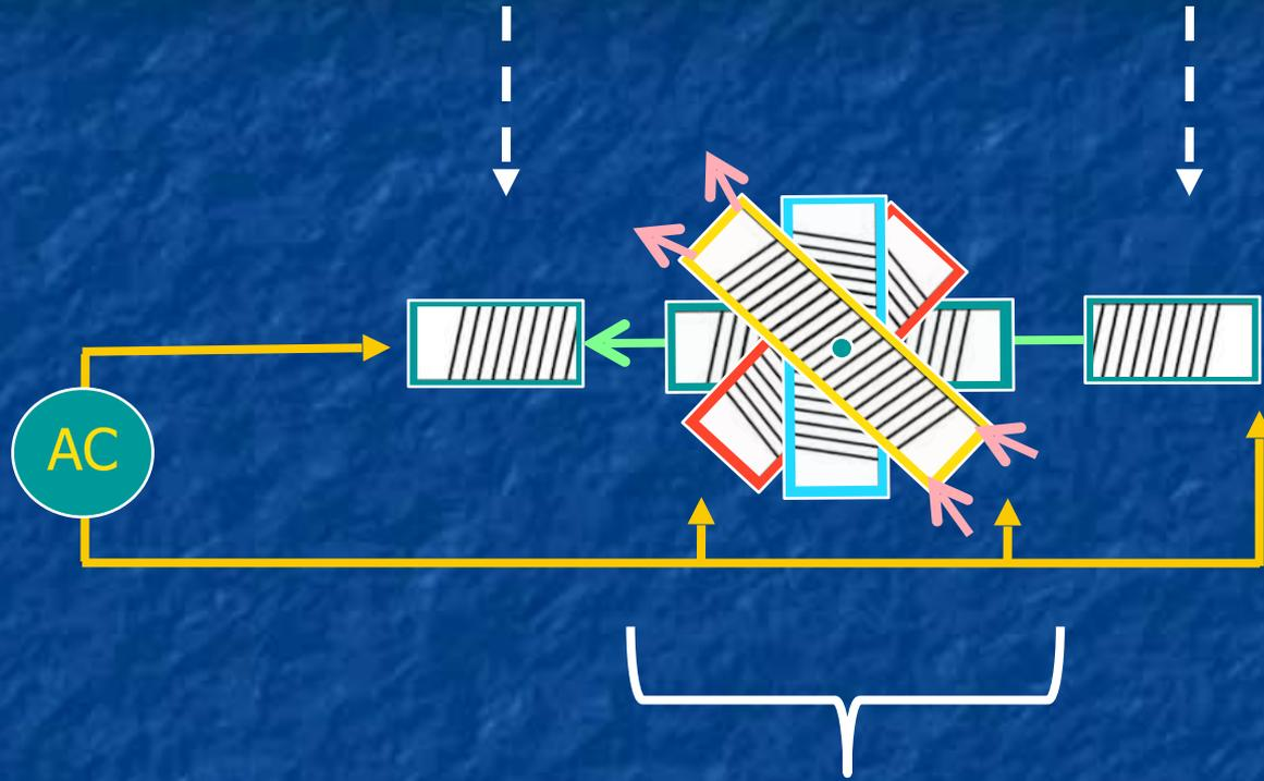
INNER ("rotor") AC electromagnets (14 rather than the 4 that I fit into drawing)
