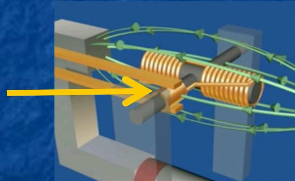
Especially split rings (which can also spark when the contacts slide over gaps)!
