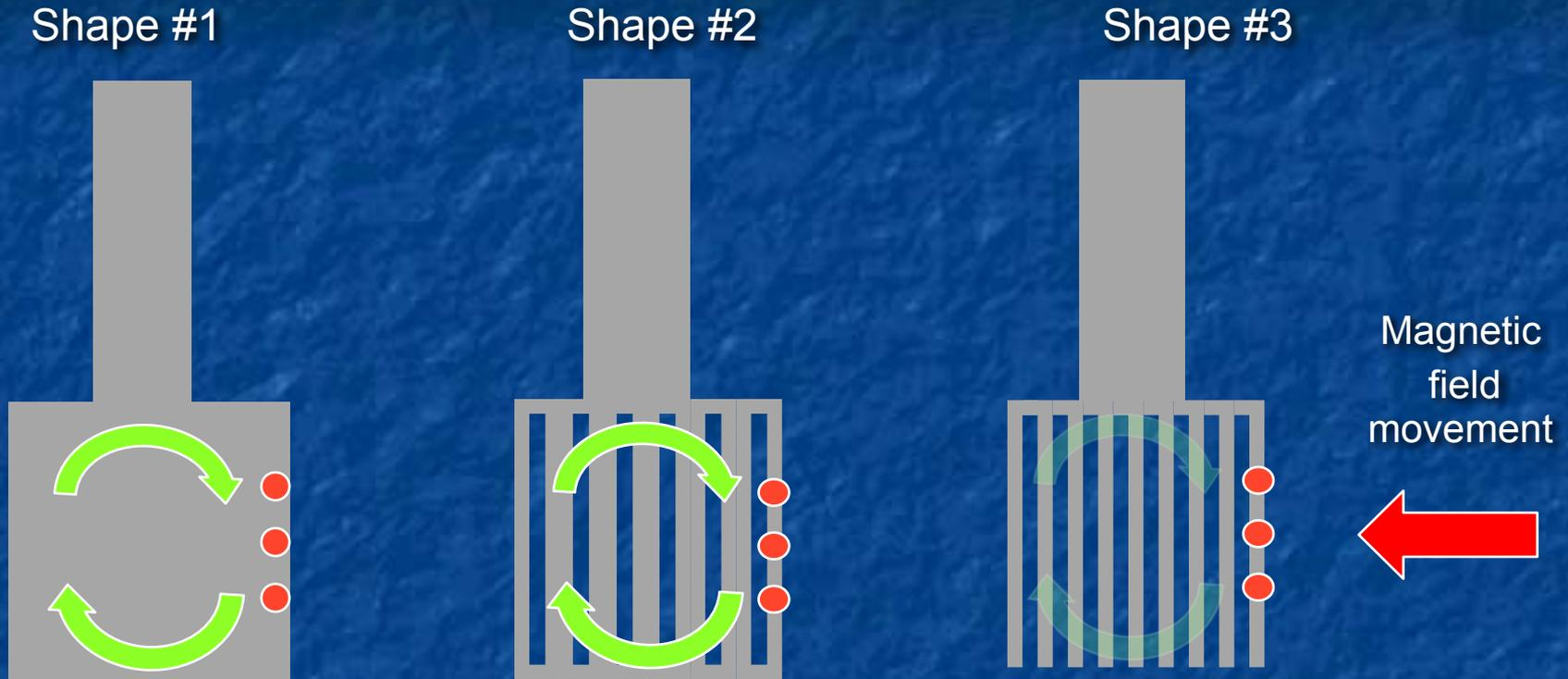
By blocking the induced electron current loops in the final comb shape
