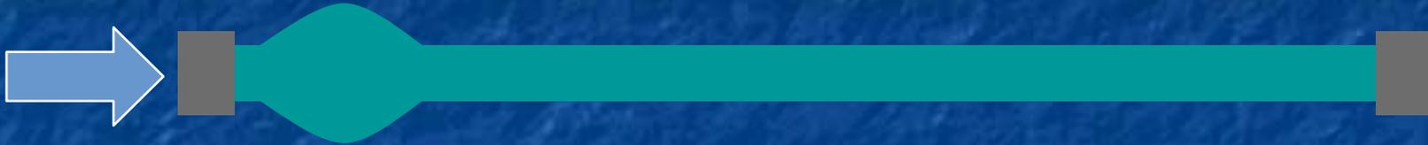
Later: Bulge has spread out, whole hose has slightly expanded due to pressure:
