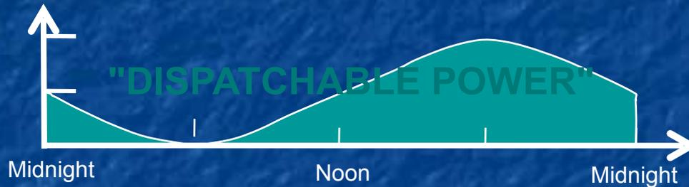
Throttling of hydroelectric or steam plants can help out a little bit
