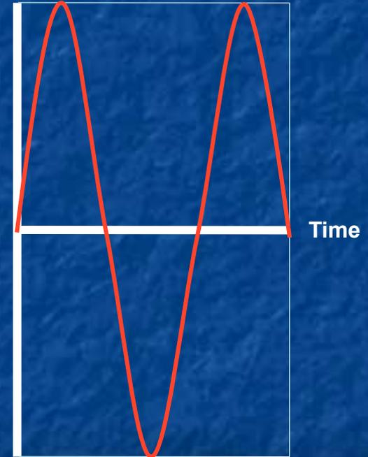
**Higher voltage out means lower current flow => Lower resistive loss**
