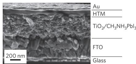
**Figure 4 |** Cross-sectional scanning electron microscopy picture of a mesoscopic perovskite solar cell prepared by the sequential deposition method. CH<sub>3</sub>NH<sub>3</sub>PbI<sub>3</sub> densely infiltrates the TiO<sub>2</sub> scaffold and forms an interpenetrating network junction on the nanometre length scale. FTO, fluorine-doped tin oxide. Figure reprinted from ref. 23, Nature Publishing Group.
