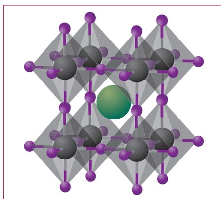
**Figure 1** | Crystal structure of cubic metal halide perovskites with the generic chemical formula  $\text{ABX}_3$ . Organic or inorganic cations occupy position A (green) whereas metal cations and halides occupy the B (grey) and X (purple) positions, respectively.
