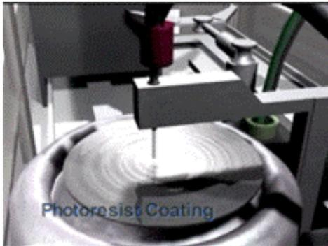
Figure 4. Frame from visualization depicting the microelectronics fabrication step of photolithography (Lucas Hardi and Matt Shields)
