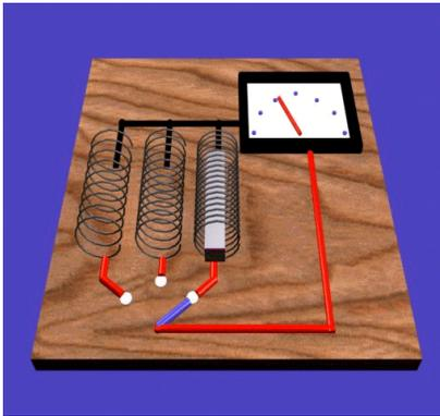
Figure 1. Frame from virtual experiment depicting electromagnetic induction (Conor Hiney)
