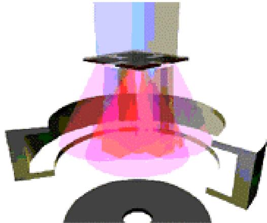
Figure 5. Frame from visualization depicting a possible future lithographic tool based on electron projection lithography (Niladri Kansari)
