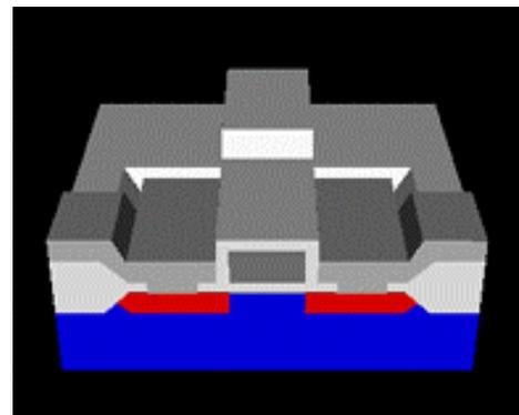
Figure 3. Frame from visualization showing fabrication of MOSFET transistor (John Bean)
