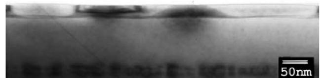
FIG. 6. Samples annealed after cold capping are also truncated if the QD height is greater than that of the average layer thickness.
