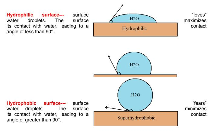
**Superhydrophobic surface** - surface has nano-scale roughness, leading to contact angle of greater than 150°.
