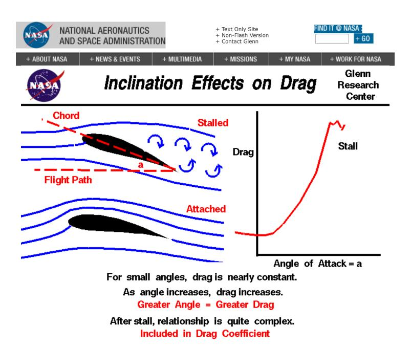
As a wing moves through the air, the airfoil is inclined to the flight direction at an angle. The angle between the <u>chord line</u> and the flight direction is called the **angle of attack** and has a large effect on the <u>drag</u> generated by the wing.
