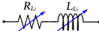
Figure 11. Equivalent electrical diagram for the lift force applied to a blade element.
