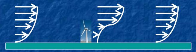
With turbines should be as tall/big as possible to capture higher speed upper winds:
