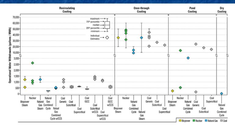
Figure 2. Operational water withdrawals for fuel-based electricity generating technologies. IGCC: integrated gasification combined cycle. CCS: carbon capture and storage.
