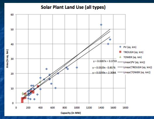
Silicon Solar PV: 0.029 km<sup>2</sup> / MW => 34 W / m<sup>2</sup>
