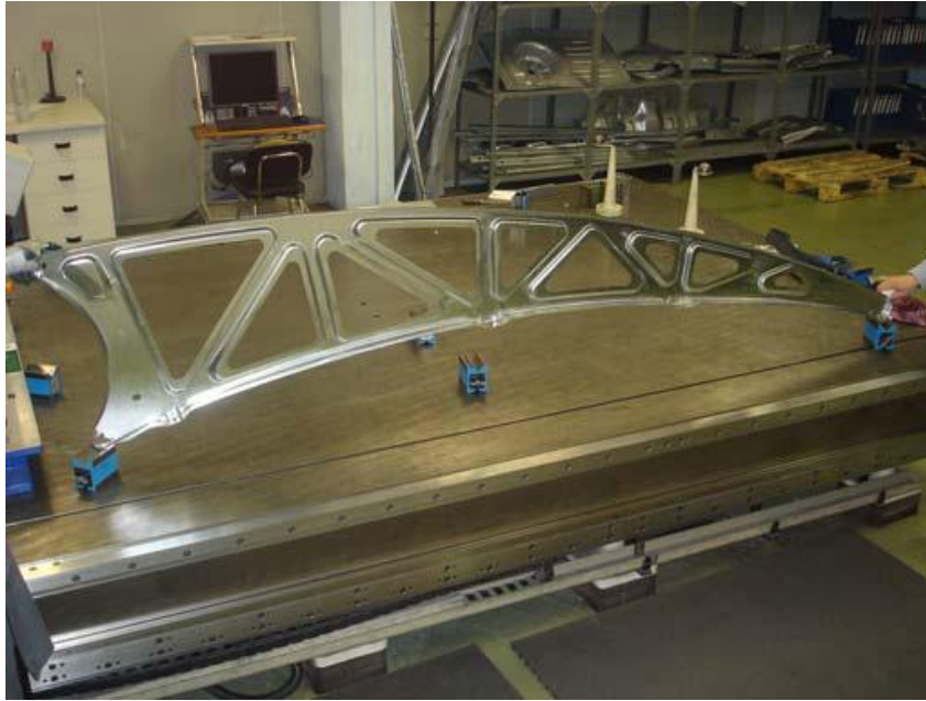
Figure 31: A stamped cantilever arm of the Senertrough (Source: Castañeda, SENER)
