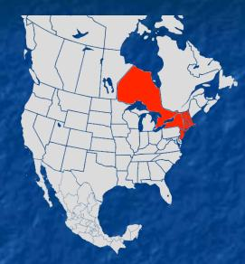
"Maintenance personnel incorrectly set a protective relay on one of the transmission lines . . . a small surge of power originating from the Robert Moses generating plant in Lewiston, New York caused the improperly set relay to trip at far below the line's rated capacity" <sup>1</sup>
