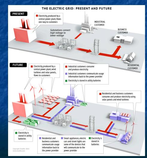
Change is instead at the ENDS of the wires: In the 5<sup>th</sup> Smart Grid feature, an Advanced Metering Interface (AMI) With the job of controlling demand, and thereby mitigating trouble At its lowest level, this consists of a Smart Meter Old power meters only recorded your total monthly power consumption Smart meters instead tell the power company what power you consumed when They also "run backward" if you produce power and send it back into the Grid
