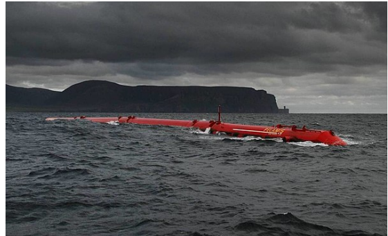
Pelamis Wave Energy Converter on site at the European Marine Energy Centre (EMEC), in 2008
