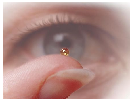
NIF's fuel "target", filled with either D-T gas or D-T ice. The capsule is held in the hohlraum using thin plastic webbing.
