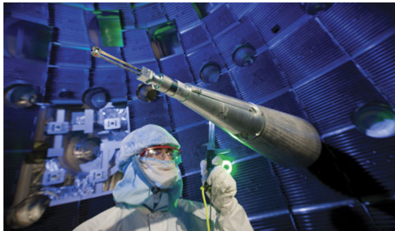
Technician works on target positioner inside National Ignition Facility (NIF) target chamber.
