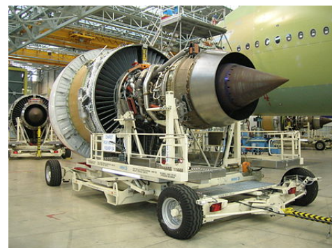
Engine Alliance GP7000 turbofan (view from the rear) awaiting installation on an Airbus A380 under construction
