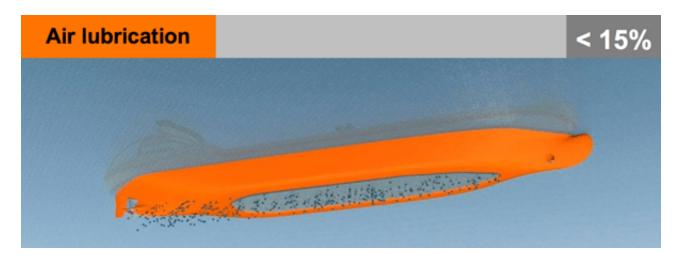
Compressed air is pumped into a recess in the bottom of the ship's hull. The air builds up a carpet that reduces the frictional resistance between the water and the hull surface. This reduces the propulsion power demand. The challenge is to ensure that the air stays below the hull and does not escape. Some pumping power is needed.
