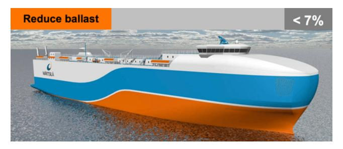
Minimising the use of ballast (and other unnecessary weight) results in lighter displacement and thus lower resistance. The resistance is more or less directly proportional to the displacement of the vessel. However there
