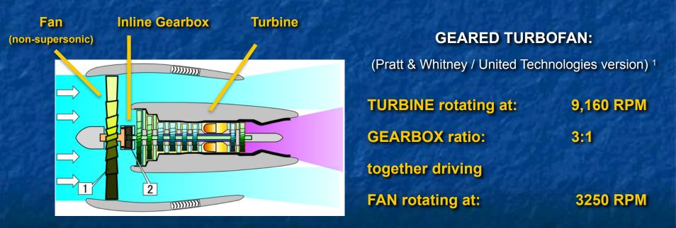
VS. earlier turboprop's 35,000 RPM turbine => 18:1 Gearbox => 1900 RPM Propeller
