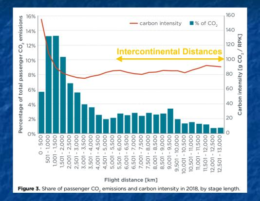
This CO<sub>2</sub> impact despite the much lower "carbon intensity" of long distance flights **Carbon Intensity** = Grams CO<sub>2</sub> per Revenue Passenger Kilometers (flown) Lower for long flights because fuel is burned **much** faster during ascent than cruising
