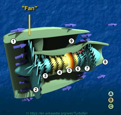
But that fan still rotates so fast that its blade tips go supersonic And their resulting mini sonic booms waste energy because their noise must be muffled by adding layers to the engine's shell (increasing M<sub>plane</sub>) and their turbulence also degrades the engine's fuel consumption / CO<sub>2</sub> emission Leading to present day proposals that they be replaced by **Geared Turbofan Engines** Which actually represent a half step back towards Turboprops:
