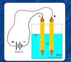
At the left negatively charged cathode: 4 H<sup>+</sup> (aq) + 4 e<sup>-</sup> => 2 H<sub>2</sub> (g) While at the right positively charged anode: 2 H<sub>2</sub>O (l) => O<sub>2</sub> (g) + 4 H<sup>+</sup> (aq) + 4 e<sup>-</sup>
