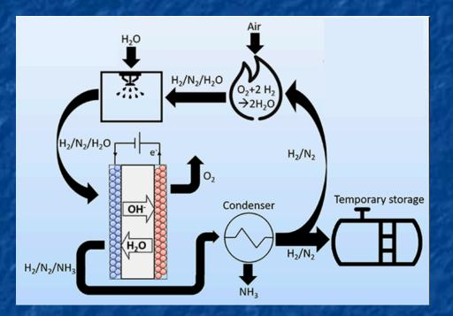
From the cathode (blue), H<sub>2</sub>, N<sub>2</sub> & NH<sub>3</sub> are piped to a condenser that separates out the NH<sub>3</sub> product while piping onward the remaining H<sub>2</sub> + N<sub>2</sub>
