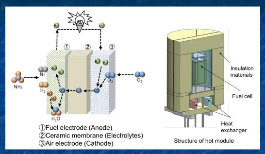
Reporting 56% efficient output above 1kW, with stable thermally independent operation
