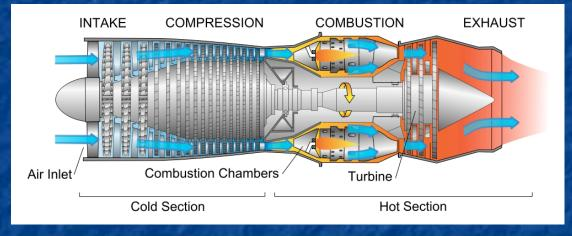
Those turbine blades were attached to shaft thereby spun by the exhaust gas At the front of that spinning shaft a series of **compressor blades** were also attached, which compressed thin incoming high-altitude air enough to maintain combustion
