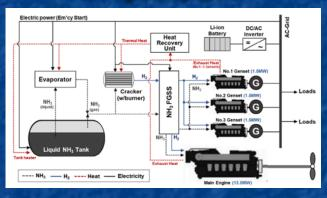
H<sub>2</sub> (from NH<sub>3</sub>) burned in ICE driving electric generators powering propellers' electric motors
