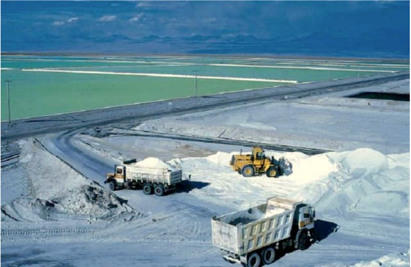
Rich brine pools containing lithium and other minerals evaporate in the Atacama desert in Chile. (Image courtesy of SQM.)
