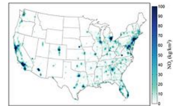
Distribution of estimated actual excess Volkswagen light duty diesel vehicle NO x emissions summed over 2008 through 2015 (kg per km 2 ). [187] The median value of emissions is used for each year. Emission density peaks at 446 kg per km 2 [187]
