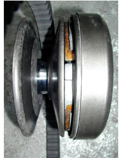
Belt-driven CVT for a motor scooter
