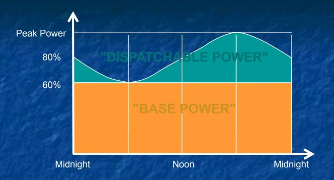
There is a **"BASE"** power demand (from 0% up to about 60% of the demand peak) On top of this is an oscillating **"DISPATCHABLE"** power demand Which cycles up from about 60% of peak, to 100% of peak at about 6 pm Which gives that ~ sinusoidal oscillation an average of ~ 80% of peak power Which also makes the **average daily power ~ 80% of peak power**
