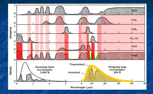
For instance: Why I have heard methane is "5X worse" or "30X worse than CO<sub>2</sub>" Because it is NOT about methane's entire absorption spectrum It's about where methane absorbs IR colors that no other gas has already absorbed And that depends on the **absorption spectra** of ALL the other gases And on the **concentrations** of ALL those other gases Making this an extremely complex and tightly interwoven calculation! Another way of looking at this is "Global Warming Potential"
