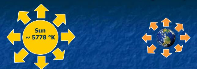
With its light spreading out, sun delivers far less power/area to earth's atmosphere Earth then re-emits that energy in all directions (not just side receiving sunlight) So balance of heat flow to and from earth' surface is achieved with earth surface temperature far less than sun's 5778 °K surface temperature And we all know balance comes with earth surface temperature of about 300 °K But that "about" is all important to those of us living on the earth!
