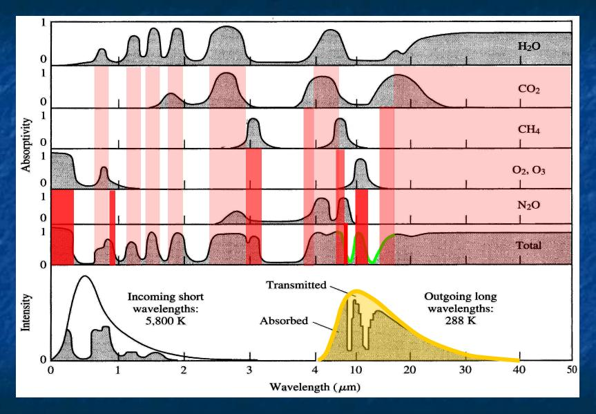
Heat loss window is now mostly shut by CO<sub>2</sub>, CH<sub>4</sub>, O<sub>2</sub>, O<sub>3</sub> and N<sub>2</sub>O
