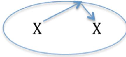
This is used in “pumped” lasers which employ long ellipsoidal mirrors. An intense flash lamp is laid along one focal line and the material to be lased along the other focal line (e.g., a tube of lasable neon or argon gas, or a ruby crystal as in the world’s first laser).
