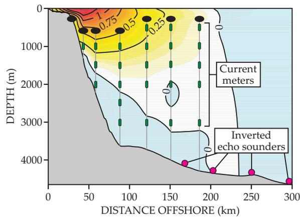
**FIGURE 2. THE INSTRUMENT ARRAY** deployed to measure the Agulhas Current consisted of strings of moored, floating current meters and four inverted echo sounders that use acoustic signals to estimate the flow profile of the water above them. The contours indicate the mean flow velocity in meters per second. (Adapted from ref. 2.)
